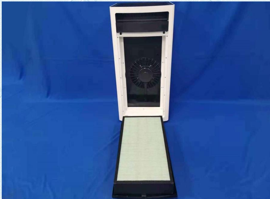
Photo 6 - Side cover and filter removed
